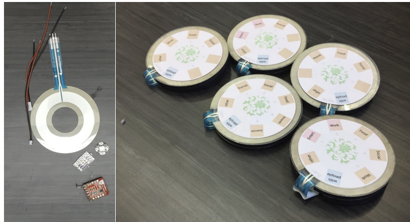
Fig 1. (Left) Individual components of each Heed device include a circular touch-sensitive soft-potentiometer, LED, a micro-controller with an integrated BLE module, and a custom designed Printed Circuit Board. (right) The Heed devices used in Study 1.
