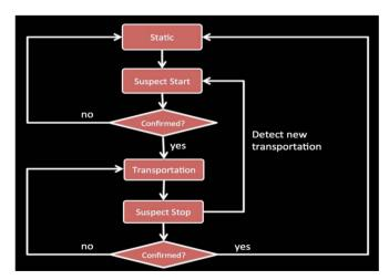
**Fig. 2.** We built a finite state machine (FSM) to process activity labels received from the Google Activity Recognition service and to determine whether a user is in a certain transportation or is stationary. The FSM has four states: Static, Suspected Start, Transportation, and Suspected Stop.
